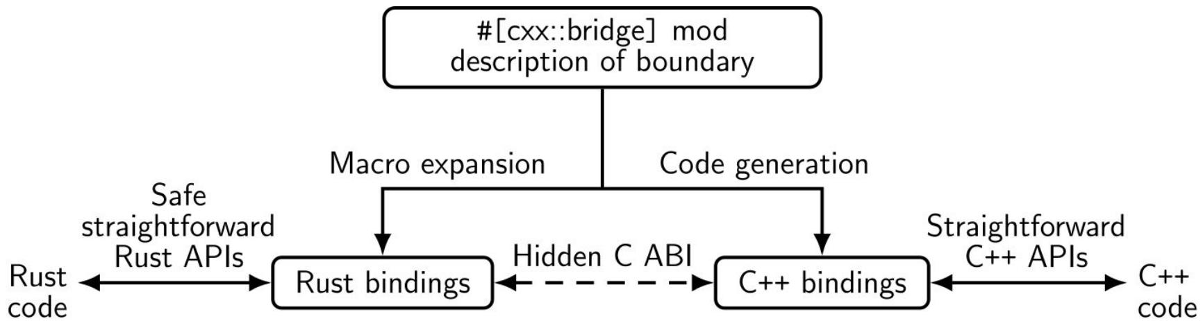
"The resulting FFI bridge operates at zero or negligible overhead, i.e. no copying, no serialization, no memory allocation, no runtime checks needed." – <https://cxx.rs>
